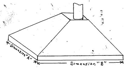
Multiply dimension "A" by dimension "B", that is the square feet of surface area. Multiply surface area by 200 FPM and that gives you the cubic feet per minute of exhaust you need.
